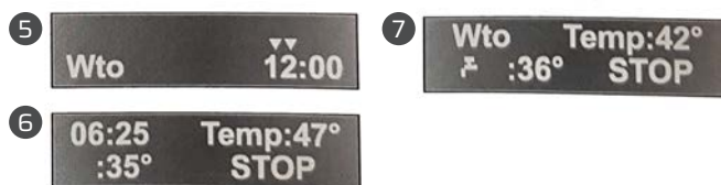
Fig. 4.9b. Furnace controller screens
